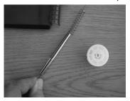
3) Pry pulley off of motor with screwdriver.
