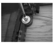
8) Discard old cable. Thread spring and latch on the new cable and pulley.
