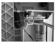
5) Pull metal latch and spring completely off the door panel.
