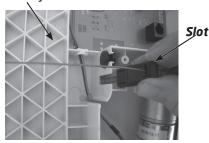
Insert the sandwiched cable guides into the guide slot of the frame just below the motor pulley.
