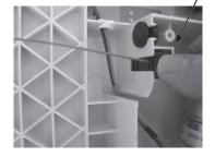
17) Finally, remove any slack in the cable by winding the pulley (turn with your fingers or pliers). Re-attach the rear frame using six flat head screws at the top of the door, and pan head screws around the rest of the door frame. Do not over tighten the screws.
