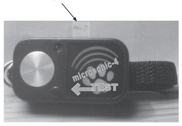
This tab is in place to protect the battery during shipping. Do not replace it.
