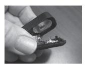
C. Replace battery in top with the metal ring visible.
