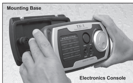
A. Separate Mounting Base From Electronics Console.
