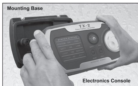
A. Separate Mounting Base From Electronics Console.
